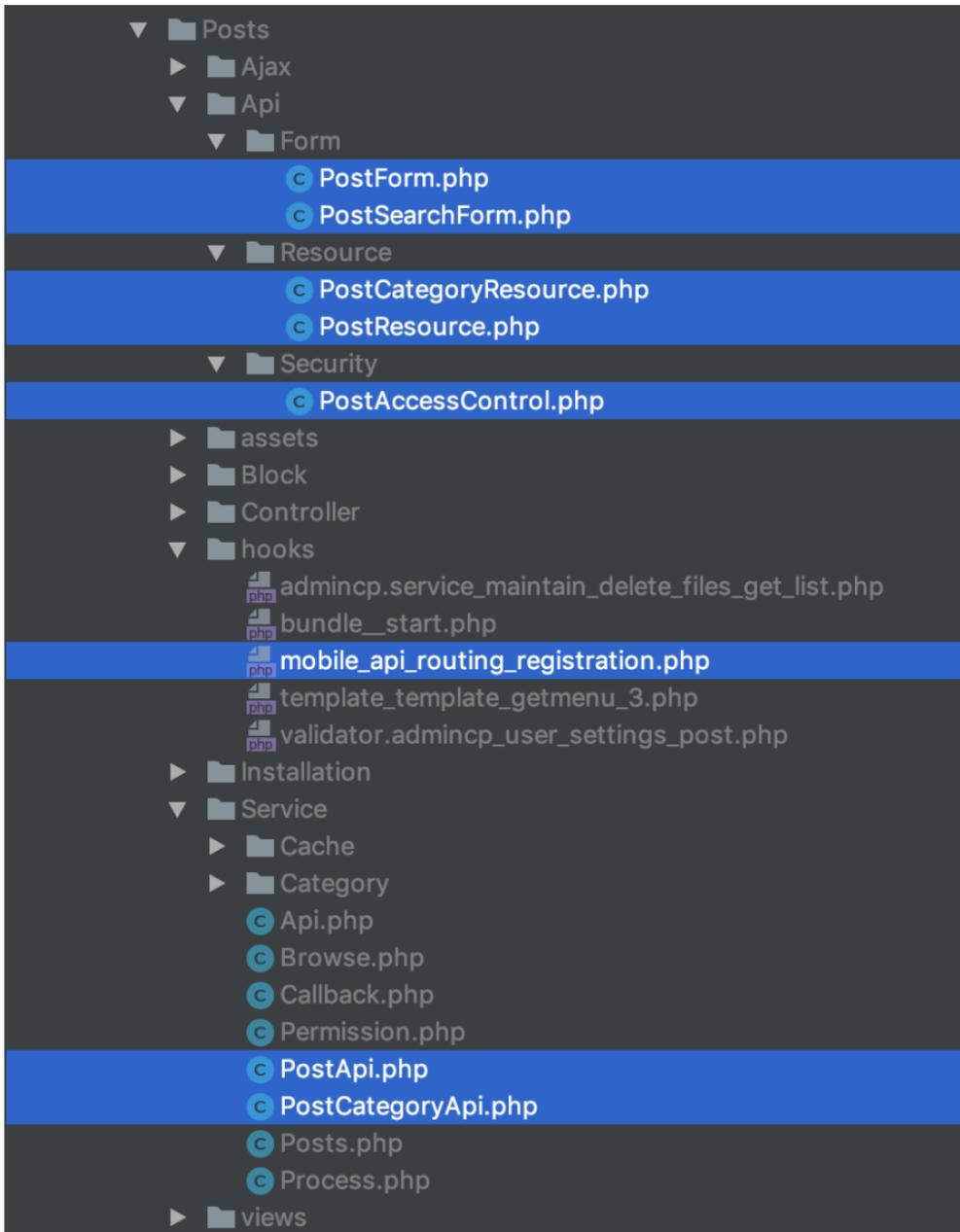
The picture above shows the basic structure to extend your app to support Core Mobile API. Take a look at highlighted items and let go to the detail of each section
